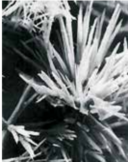
Picture 9: Lime protective layer
