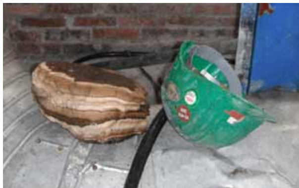
Deposit removed from pipe after Vulcan installation
