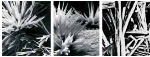
Picture 9 Lime protective layer
